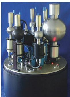
ROSPEC<sup>TM</sup> is a rotating neutron spectrometer manufactured by BTI
