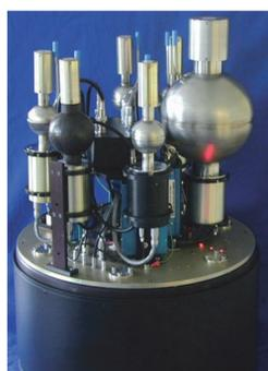
ROSPECT<sup>TM</sup> is a rotating neutron spectrometer manufactured by BTI
