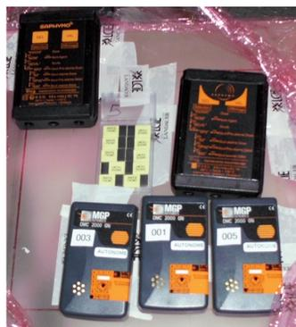
Positioning of the dosimeters on the slab phantom
