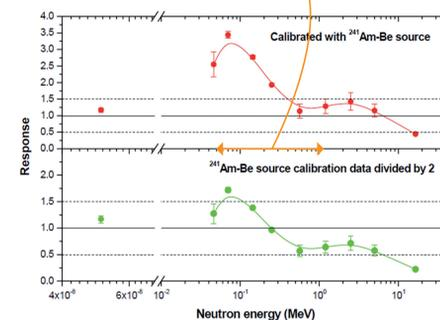
Energy response of the Neutrak. In the range of 50 keV to 1 MeV, the energy response of the Neutrak meets the ISO 21909 standard requirements. Therefore, the Neutrak dosimeter is appropriate to use in the Chinon NPP.
