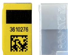
Neutrak<sup>®</sup> T (CR-39), passive dosimeter with fast neutron and thermal neutron detectors (LANDAUER Product)
